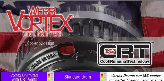
These infra-red photos taken on the Webb dyno show a Webb Vortex Unlimited drum with CRT vents next to a standard drum at precisely the same moment during the braking cycle. Compare the heat (red color) and you can actually see that Vortex runs significantly cooler.
